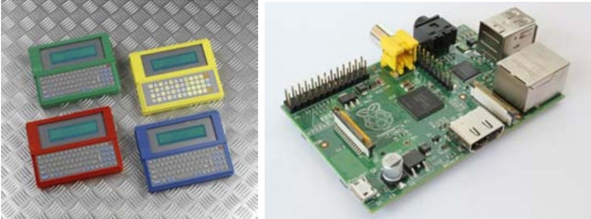
The Camdata Raspberry terminal consists of a Raspberry Pi Computer board fitted into the Microscribe T4000 terminal enclosure. The terminal is battery powered, but can be powered from an external power adapter (batteries will be required to maintain the Real Time Clock operation).
